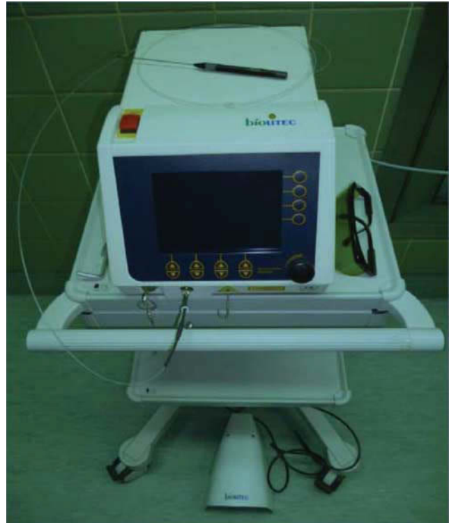
Diode laser of 980-nm wavelength with a fibro-optic delivery system (Ceralas D25, 980 ± 30 nm, 25 W, model 003; CeramOptec GmbH, a company of Biolitec Group).
